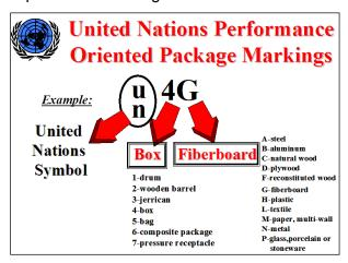
The markings on the outer container surfaces could be different for certain types of packages. All UN POP markings are permanently marked on the container. Handwritten marks are not authorized under the UN recommendations. The most common POP that is offered to FedEx Ground is the fiberboard box.
